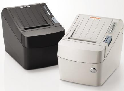
The SRP-370 is a super-high-speed thermal receipt printer that can print 200 mm per second, and has been made for wider applications including ticketing, lottery, and kiosk as well as the existing retail and hospitality industries. The SRP-370 can accept 103 mm papers for those applications, and paper replacement period has been improved by 50%. Two-color printing is also supported so that receipts for various promotional purposes can be printed.
